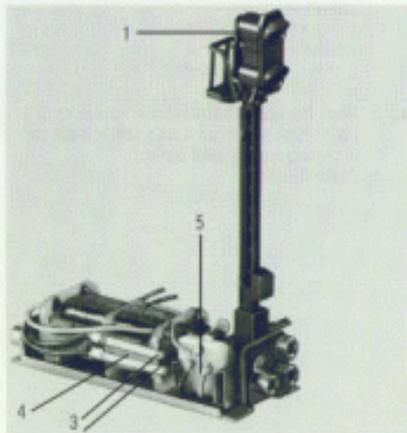
The contact plate (1) is not correctly clipped into place or is broken.
