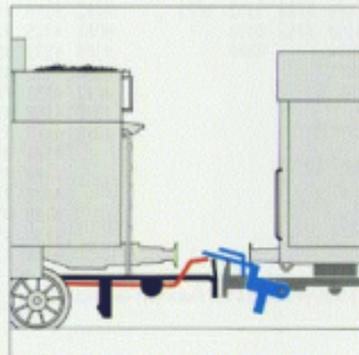
Several Märklin locomotives are equipped with the TELEX coupler. These units can be found in the current HO catalog. These locomotives can be uncoupled from their cars at any spot on the layout by remote control at the transformer.
