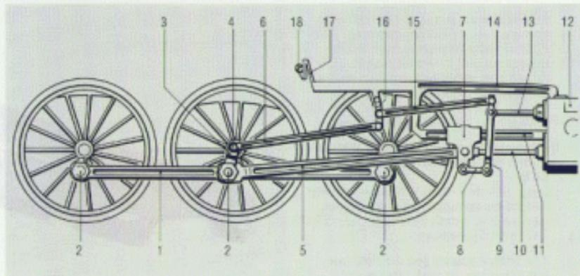
**b.....** If the combination lever (9) and the union link (8) are hanging behind the cross head (7) (instead of in front), the eccentric rod (6) will become jammed.
