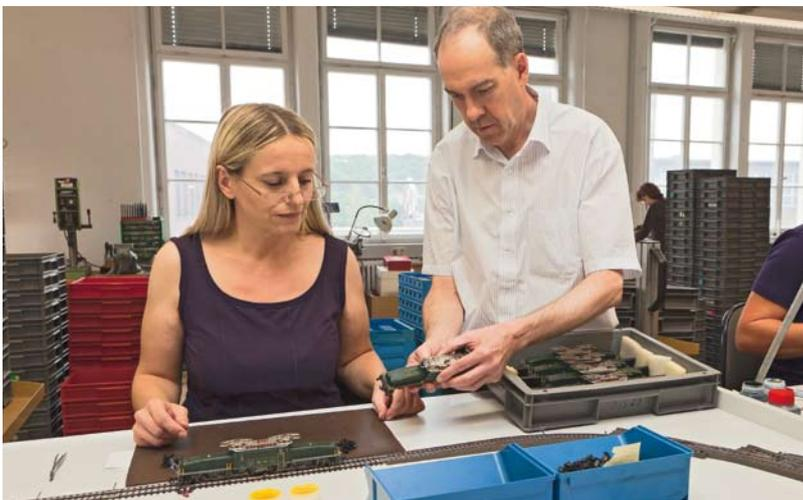
... monitors speed, direction of travel, current consumption and special and sound functions. Then afterwards, there is a visual inspection of the fittings and the paintwork.
