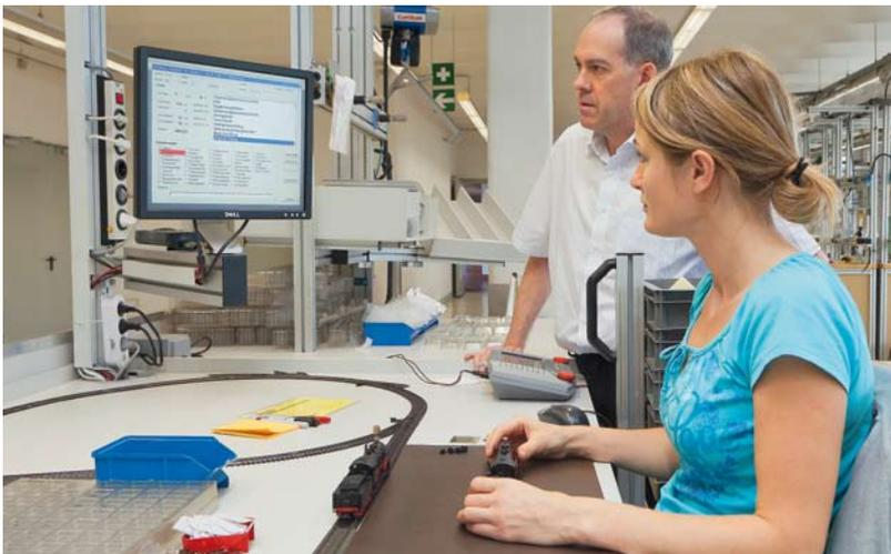
**Boundary values:** in the final inspection, the screen betrays whether functions of loco and tender are outside the narrow tolerance zone. The testing program, designed for the specific article,...
